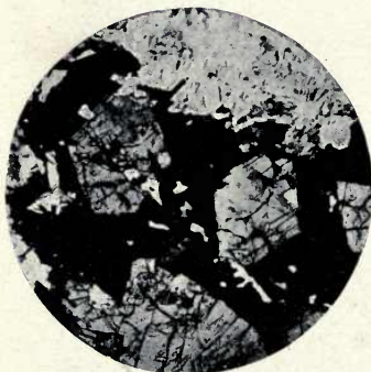
3.—Epidote. Ordinary Light. Showing form and cleavage.
